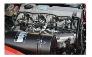
The high pressure common rail electronic-controlled engine which adopts high pressure multiple injections technology to ensure the strong power take-off, lower emission and better cold starting performance; saving the 10% of energy consumption.
