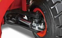
2. 2.0~3.8t roller bearing on the steering axle king pin adopts large size tapered roller bearing (TRB), larger steering cylinder and bumper block assemblies on the top, which can prolong the service life of bearing and highly improve the reliability of steering axle.
